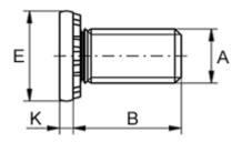
Head diameter E = 8.5Head height K +/-0.02 = 1.50Hole diameter +0.1 = 5Length B +/-0.4 = 20Male thread A = M5Min distance to edge = 10.5Tightening (N m) = 6.0
